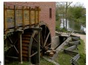
turning waterwheel to gears inside the mill which run the grinding stones.
